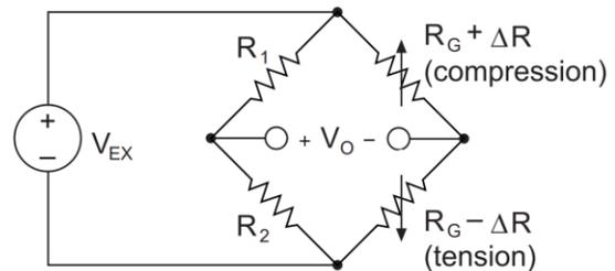
**Figure 6. Half bridge circuit**
