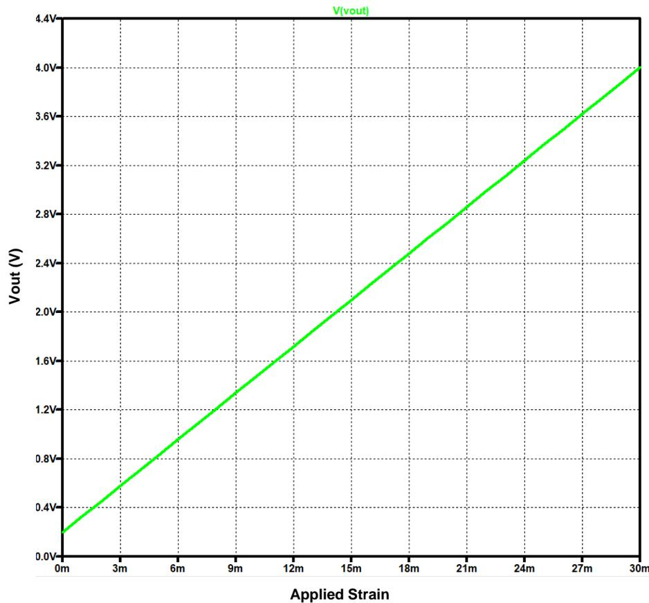
Figure 9. Plot of simulated output voltage versus applied strain in a practical half bridge application circuit of Figure 9
