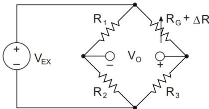
**Figure 4. Quarter bridge circuit**
