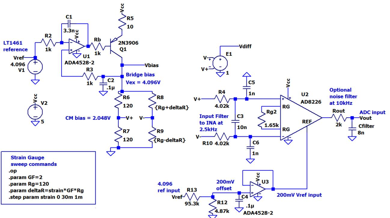
Figure 8. Half bridge application circuit showing excitation and signal conditioning circuit
