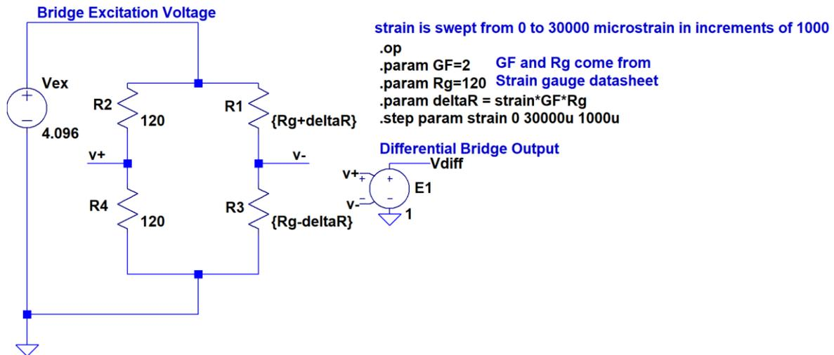
Figure 7. Schematic showing ideal half bridge model and simulation parameters
