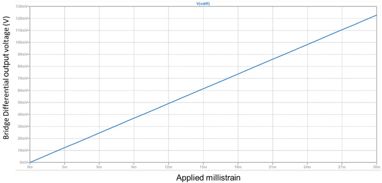
**Figure 8. Plot of simulated voltage versus strain (millistrain) using ideal sensor model and 4.096V excitation voltage**
