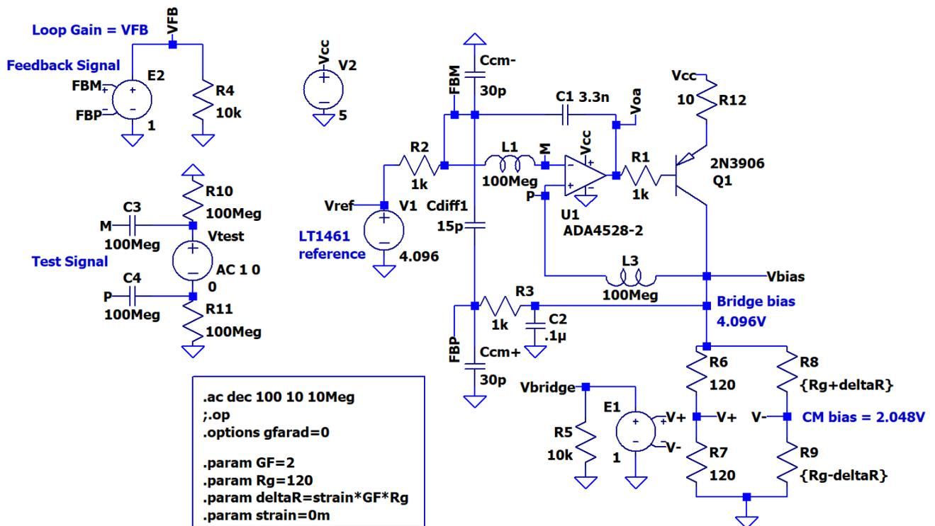
Figure 11. Bridge excitation voltage circuit loop gain analysis for stability
