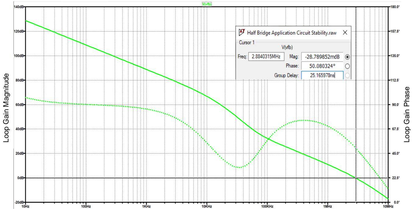
**Figure 12. Bridge excitation reference voltage loop gain and phase**
