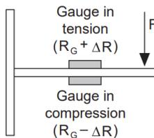
**Figure 5. Two strain gauges double the bridge sensitivity**
