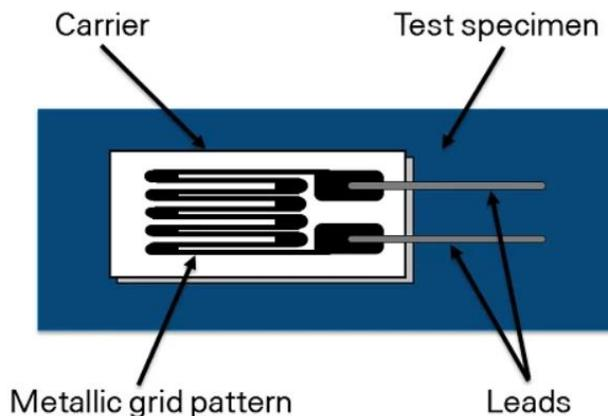
**Figure 2. Bonded metallic strain gauge**
