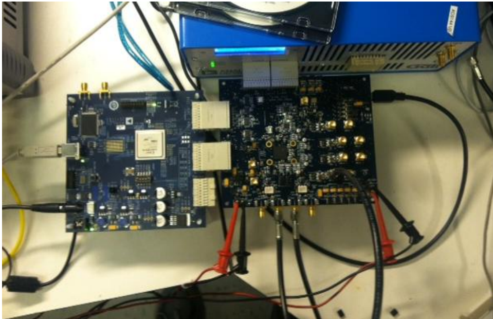
Figure 3. AD9993-EBZ Connected to HSC-ADC-EVALCZ and DPG3
