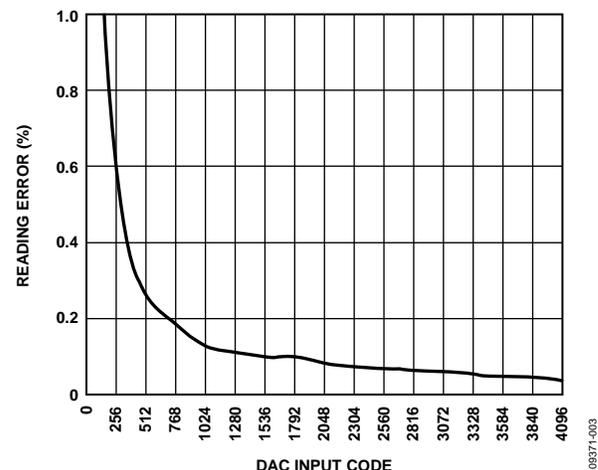
Figure 3. Output Current Error Plot
