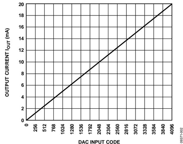
Figure 2. 0 mA to 20 mA Output Current
