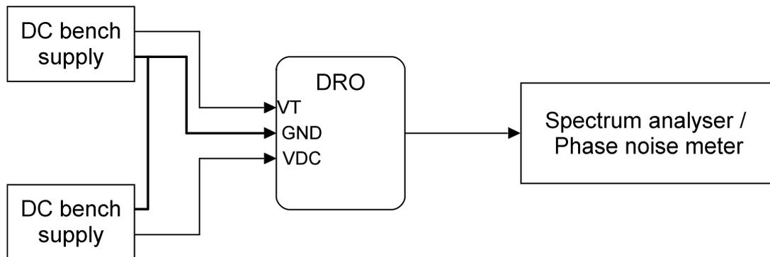
*Test setup block diagram*
