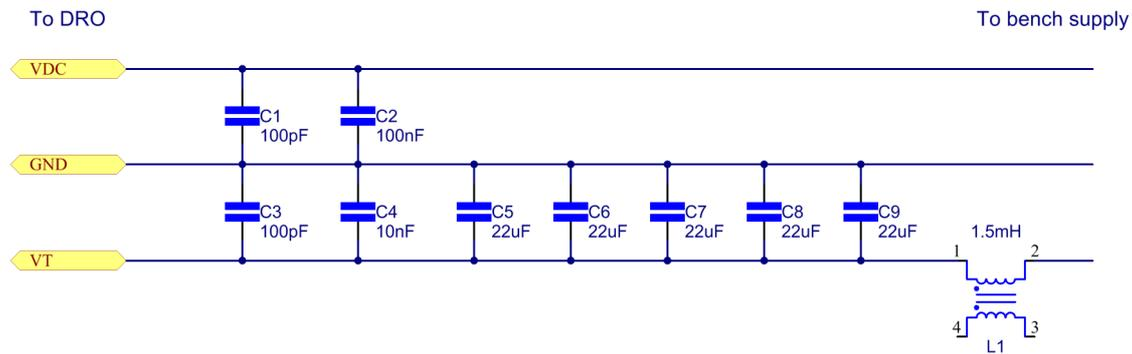
*Decoupling PCB circuit diagram*
