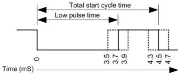
Figure 3: CEC start bit timing
