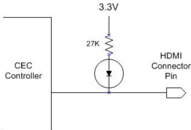
*Figure 10: Pull-up circuit for CEC line*
