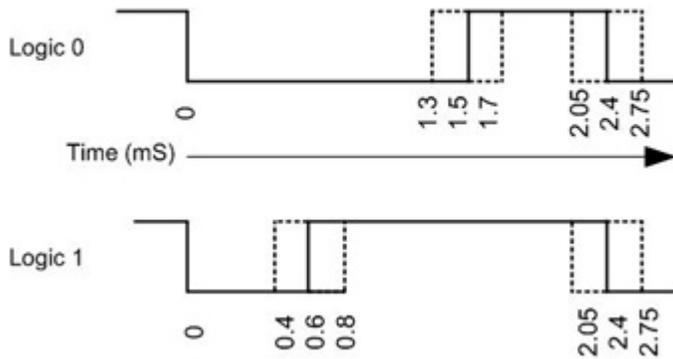
Figure 4: CEC logical state timing diagram
