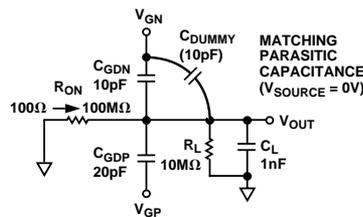
Figure 13. Matching parasitics at  $V_{SOURCE} = 0$  V (ground).
