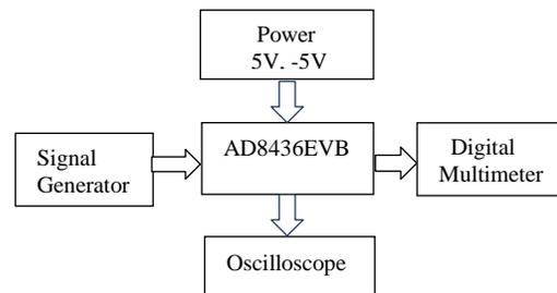
*Figure 1. Testing System Frameworks*
