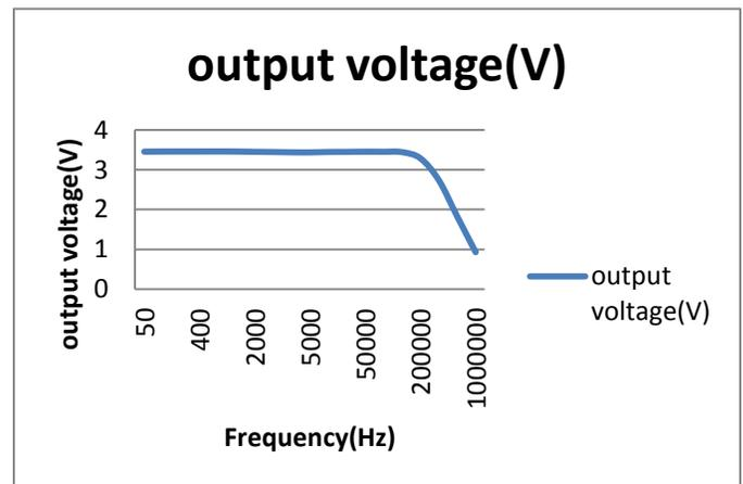
Figure 3. output voltage vs. input frequency
