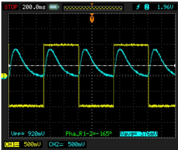
Figure 11. Input frequency is 1Hz
