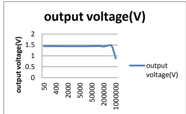
Figure 7. output voltage vs. input frequency
