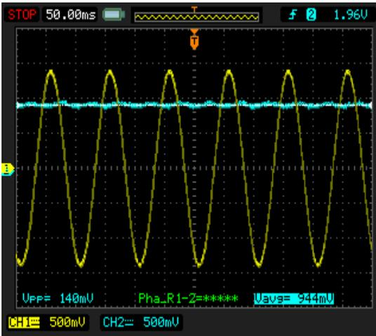
Figure 5. Input frequency is 10Hz
