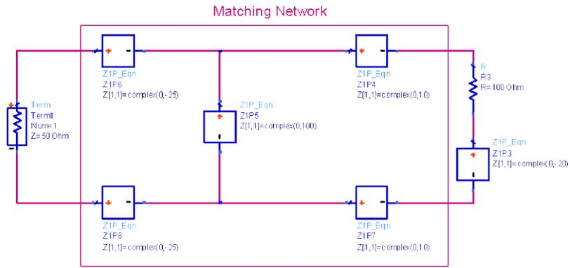
Figure 5. SEDZ Impedance Matching Schematic 3. The "T" Matching Network
