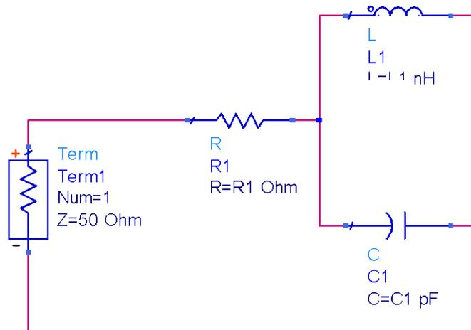
Figure 1. Series Equivalent Differential Impedance (SEDZ)
