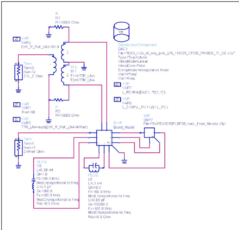
Figure 19. System Simulation Model Example – RF Connections.
