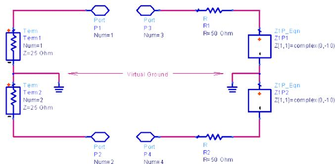
Figure 4. SEDZ Impedance Matching Schematic 2. Bisected network.
