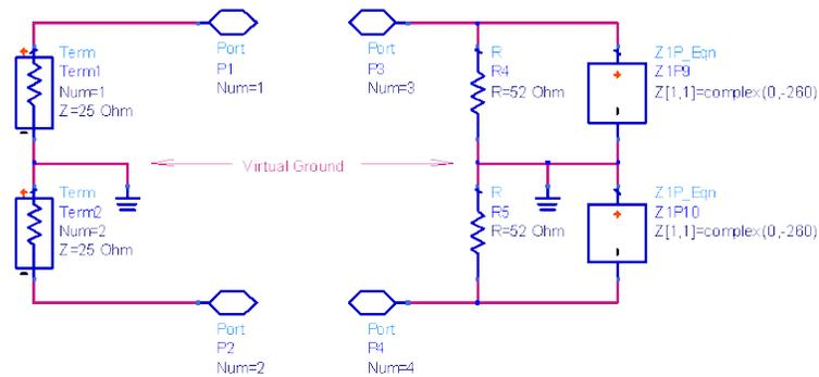
Figure 7. PEDZ Impedance Matching Schematic 5. Bisected network
