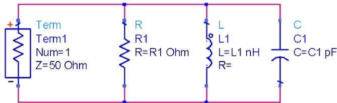
Figure 2. Parallel Equivalent Differential Impedance (PEDZ)
