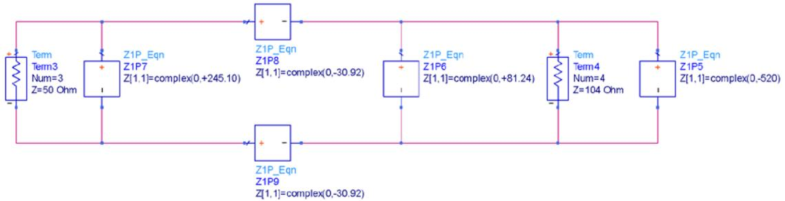
Figure 12. PEDZ Impedance Matching Schematic 10. The High-Pass Differential "PII" Matching Network.
