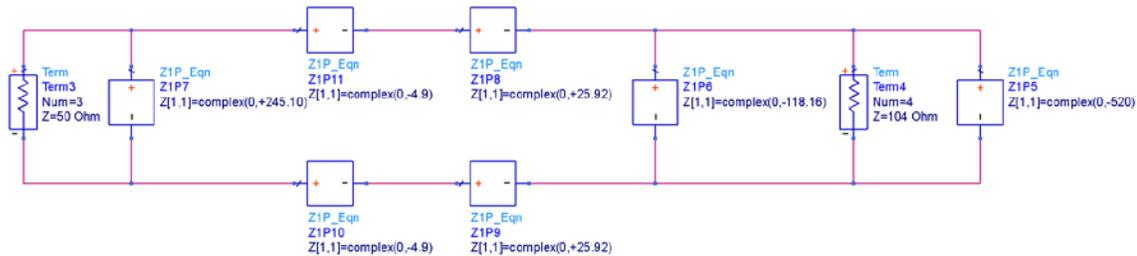
Figure 14. PEDZ Impedance Matching Schematic 12. The Band-Pass 2 Differential “PII” Matching Network.
