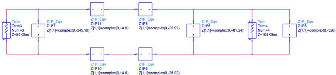
Figure 13. PEDZ Impedance Matching Schematic 11. The Band-Pass 1 Differential “PII” Matching Network.
