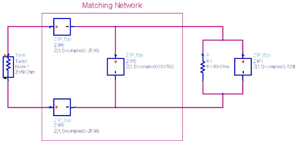
Figure 8. PEDZ Impedance Matching Schematic 6. The High-Pass Differential Matching Network
