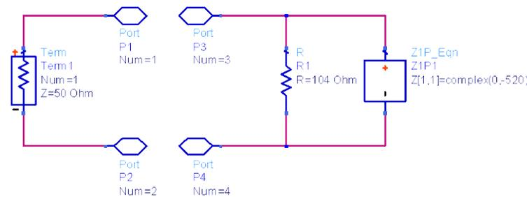
Figure 9. PEDZ Impedance Matching Schematic 7.
