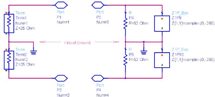
Figure 10. PEDZ Impedance Matching Schematic 8. Bisected network.
