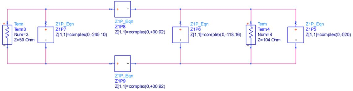
Figure 11. PEDZ Impedance Matching Schematic 9. The Low-Pass Differential "PII" Matching Network.
