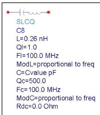
Figure 17. LEE Capacitor Model Example
