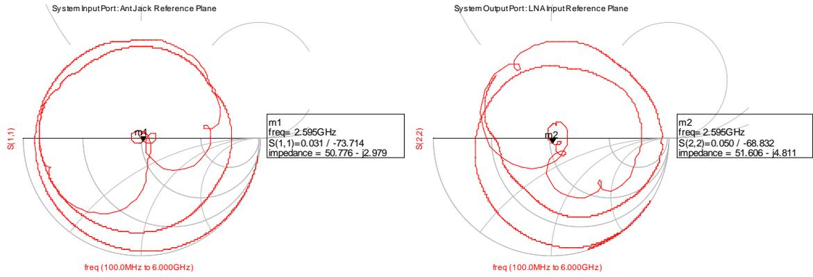
Figure 21. System Simulation Results – Post Optimization Port Reflection Coefficients.
