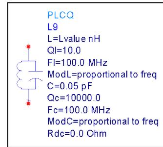
Figure 18. LEE Inductor Model Example
