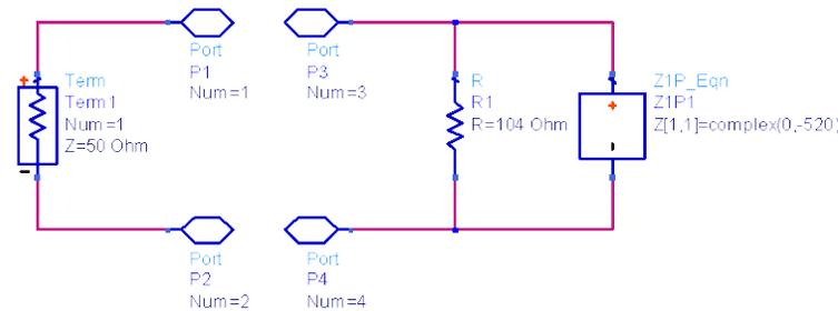
Figure 6. PEDZ Impedance Matching Schematic 4
