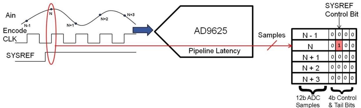
Figure1. A SYSREF± Control Bit is Used to Timestamp the Same Analog Sample that is Coincident with a Sampled SYSREF± Edge by CLK±
