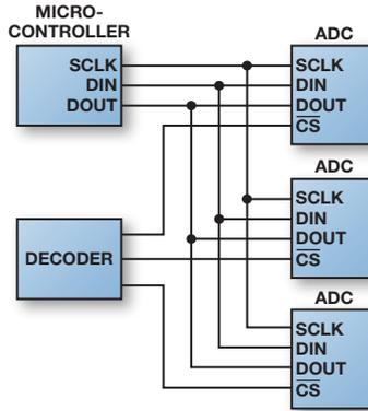
Figure 1. Interfacing several ADCs to a single microcontroller.
