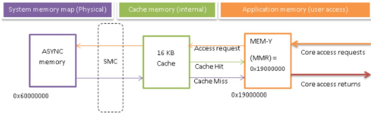
Figure: Transfer path for SMC access via Cache
