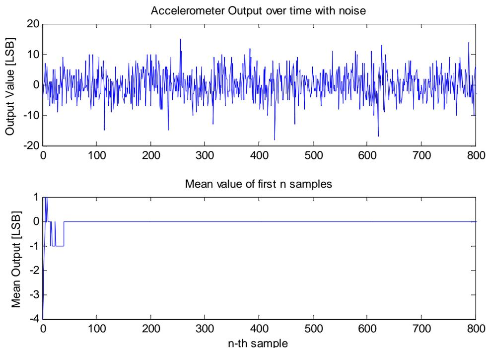
Fig. 1. Effects of filtering accelerometer output to obtain true offset value
