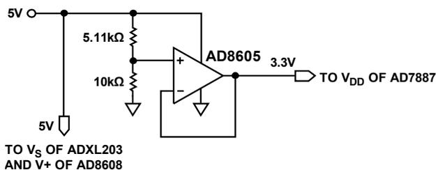
Figure 12.  $V_{\text{DD}}$  Supply for AD7887 for Ratiometric Operation
