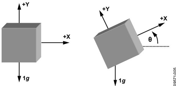
Figure 5. Two Axes Used for Tilt Sensing
