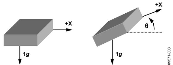
Figure 3. Single Axis Used for Tilt Sensing
