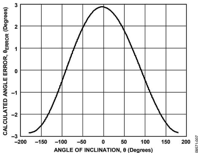
Figure 7. Calculated Angle Error Due to Accelerometer Offset
