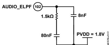
Figure 1. Audio PLL Loop Filter
