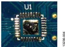
Figure 4. Tinned LFCSP Pads
