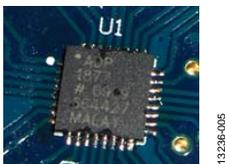
Figure 5. IC Soldered to Pads
