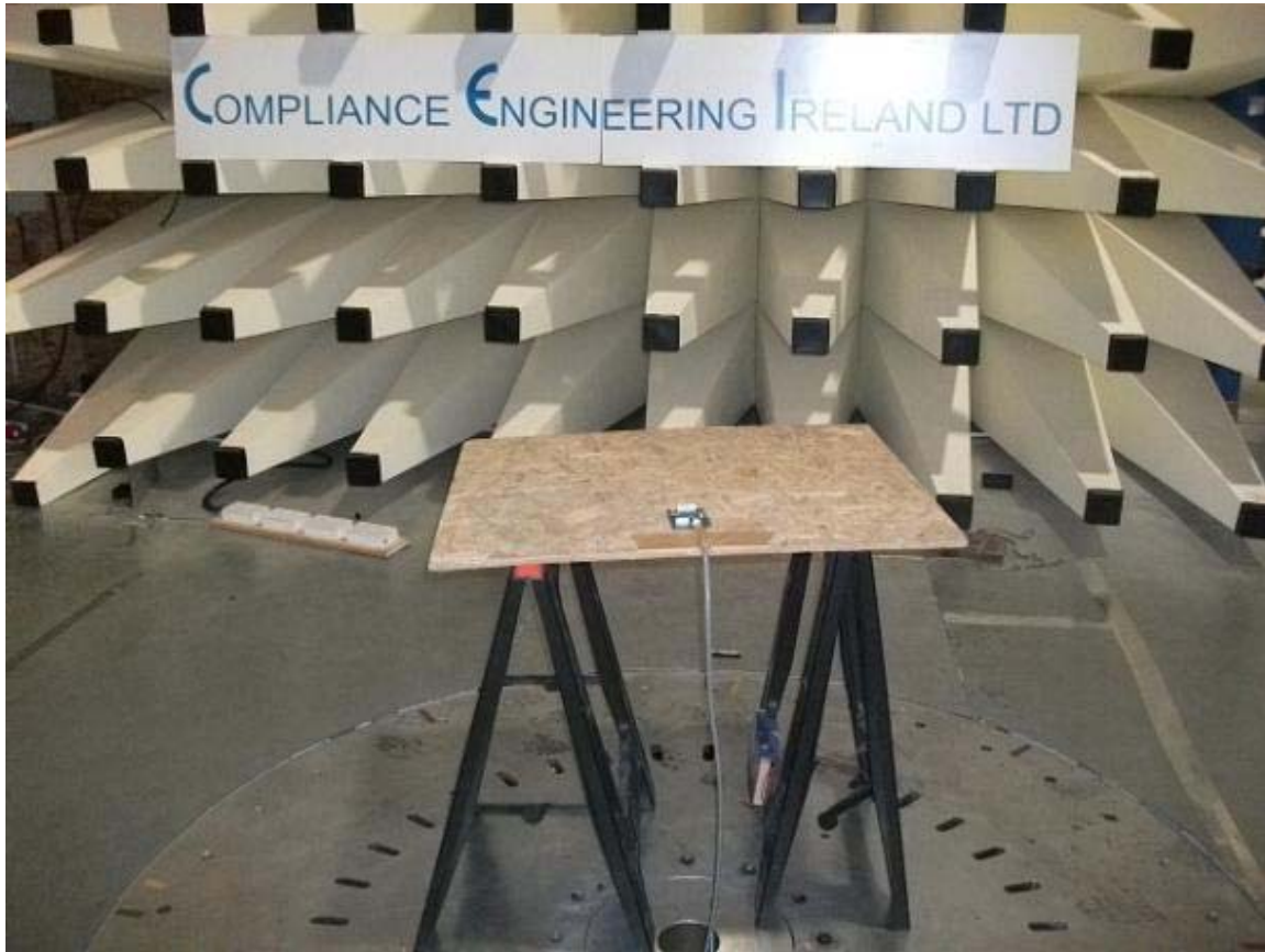
Figure 1: Radiated Emissions Test Set up
