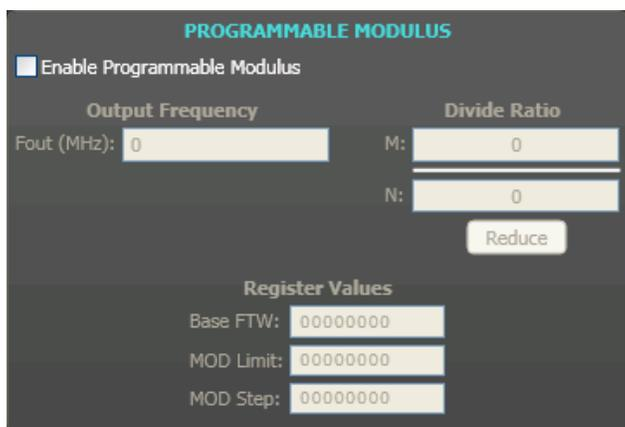
Figure 13. Programmable Modulus Window
