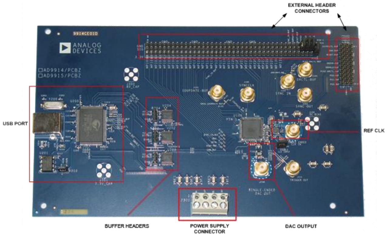
Figure 2. AD9915 PCB Evaluation Board
