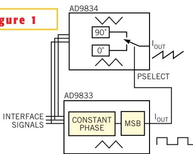
**Two DDS chips provide a convenient way to generate sawtooth waveforms.**
