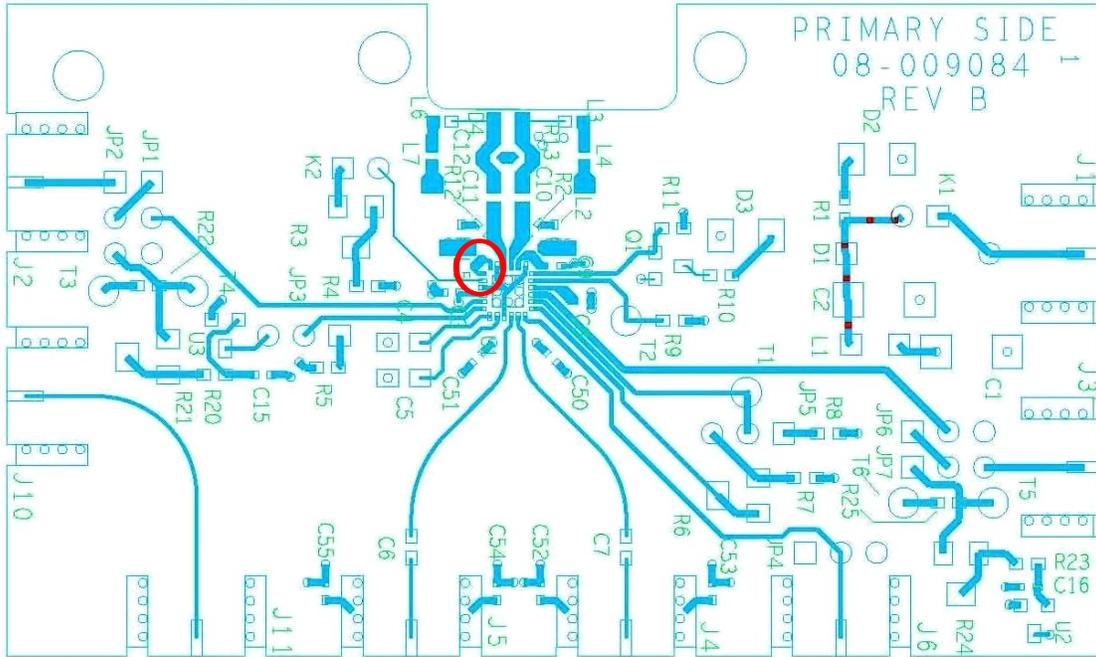
In the latest revision D, the PCB offers one option to cut off the BIAS and CCBIS pin connection. At the Red circled place, one 402 surface mount pad designed in between the pins BIAS and CCBIS. If populated DUT is ADN2871, an 0 ohm resistor is needed to connect BIAS and CCBIAS pins. If the DUT is ADN2873, leave this component pad OPEN, and the pad offers test points for BIAS and CCBIAS pins, respectively.
