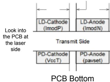
As a default setting of the EVALZ-ADN2871/ADN2873 board, the laser diode driver (DUT) to a laser diode (LD) interface circuit been optimized to work with a VCSEL TOSA: HFE4192-582.
