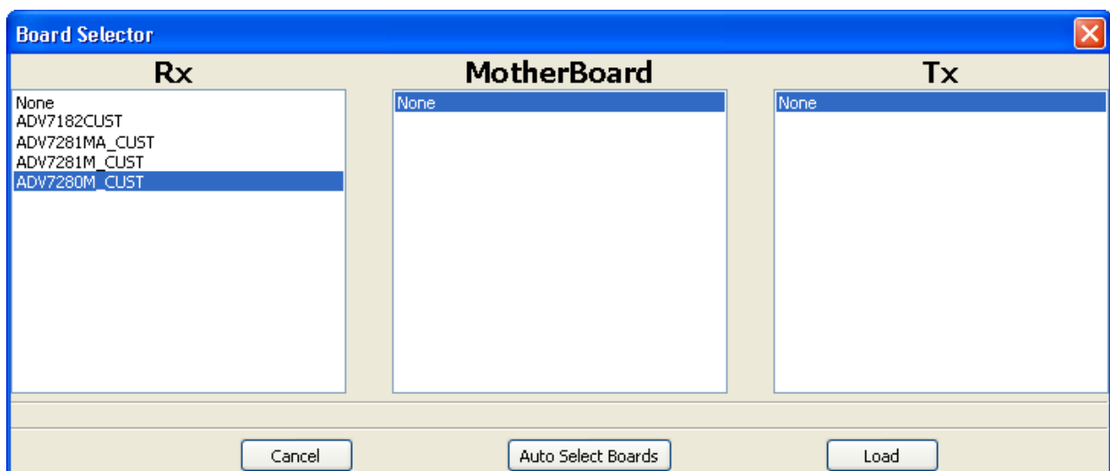
Figure 5. Board Selector Window of DVP Eval Program
